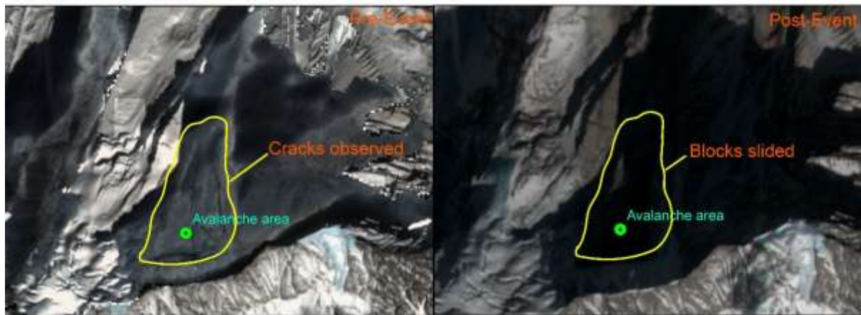
Figure 6: Pre (5 th February, 2021) and Post image (10 th February, 2021) where the cracks in the pre and the post avalanche in the Sentinel 2 image are obvious
